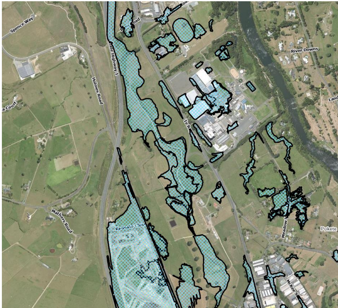
Figure 37: Current flood depression data, central Te Rapa catchment (blue hatched area shows extent of 100-year ARI flood depression).
